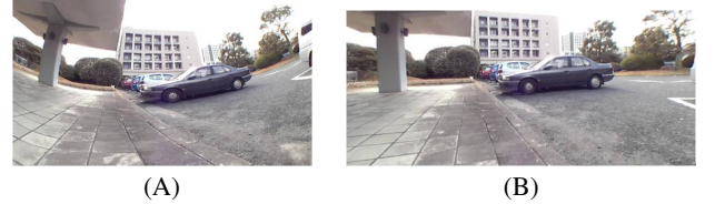
Figure 11: A result of image unwarping (perspective). (A) Input image (B) Corrected image
