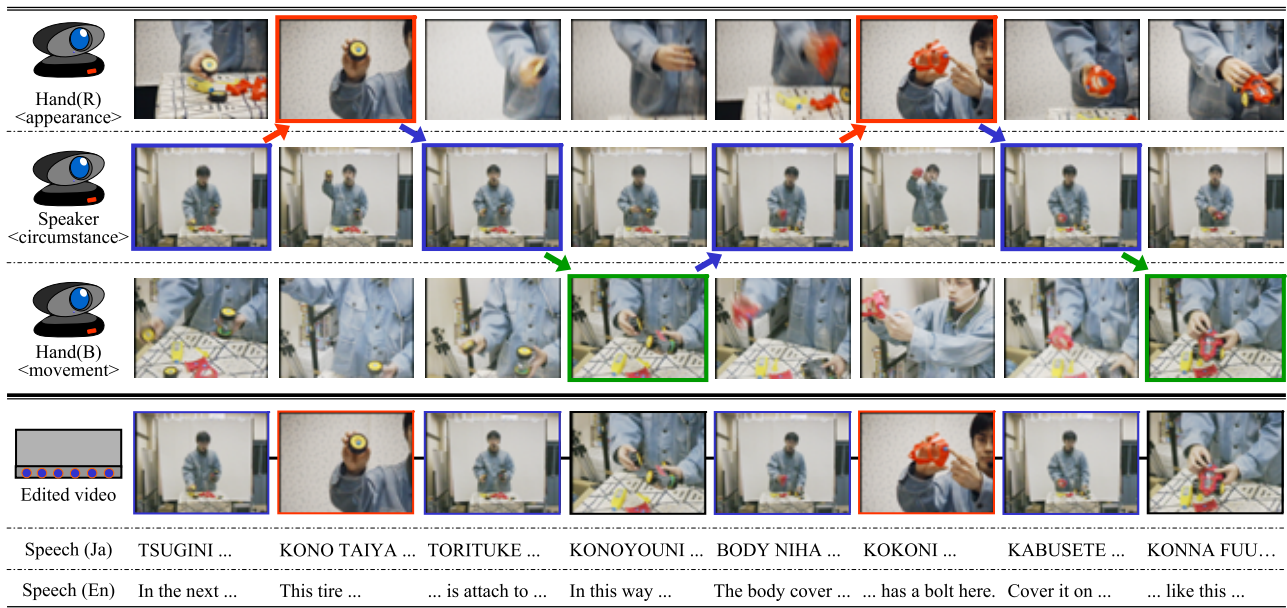
FIGURE 8 - Shot samples captured by the cameras and an example of an edited video. Hand(R) means the right hand, and Hand(B) means the left hand. The phrases below the images are the transcribed speech. The upper line shows the actual speech in Japanese, and the lower shows the translation into English. The sample movies (mpeg format) can be obtained at http://www.image.esys.tsukuba.ac.jp/~ozeki/e_movies.html .
